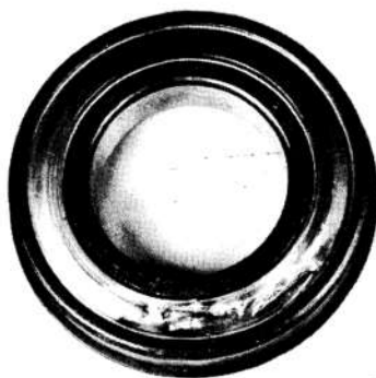
BEARING REMOVED WITH PUNCH, DAMAGED SHIELD.
