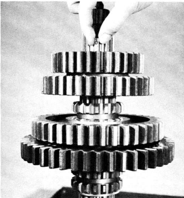
22. Align the large notch of the washer with the keyway and install the key, fitting the tapered end in the washer notch and the pin in the hole in the keyway.
