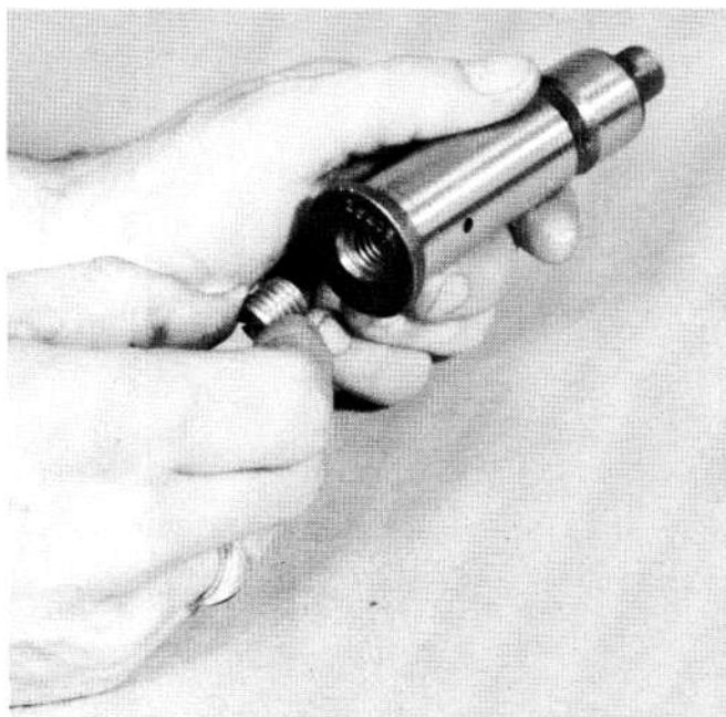
1. Install the plug in the idler shaft.
