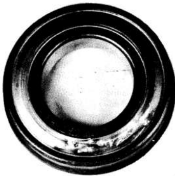
BEARING REMOVED WITH PUNCH, DAMAGED SHIELD.
