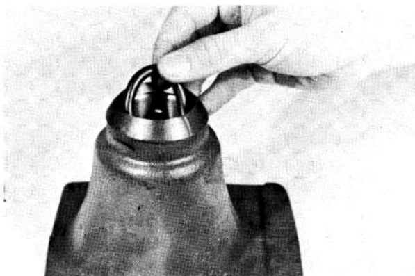
1. If so equipped, install the O-ring in the top of the housing.
