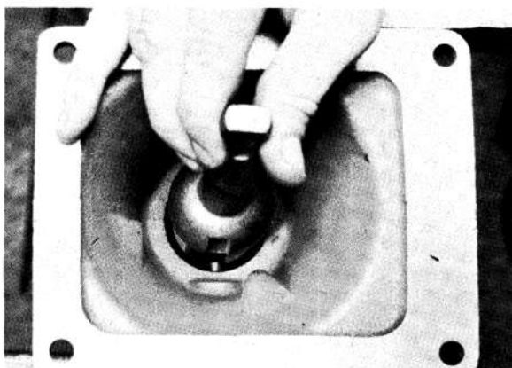
3. Install the housing in a soft-jawed vise with the bottom facing up and insert the shift lever in the housing, fitting the slot in the pivot ball of the lever with the pivot pin.
