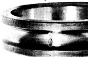
SPALLED BEARING— EXTREME LOAD
