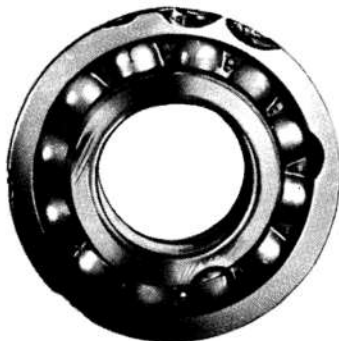
BEARING REMOVED WITH CHISEL, DAMAGED OUTER RACE.
