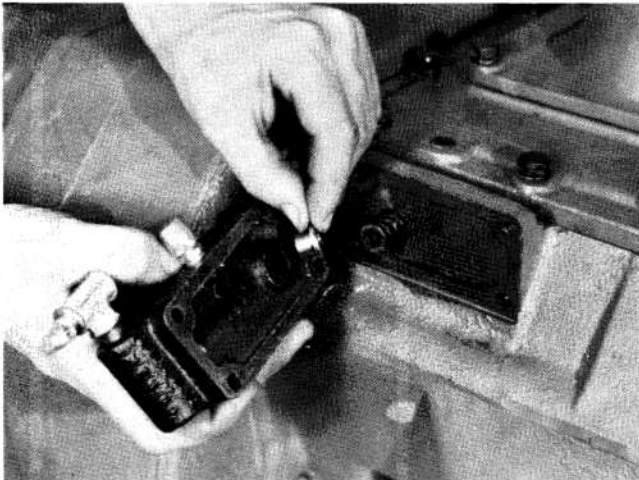
2. Install the hat-type alignment sleeve in the air valve.
