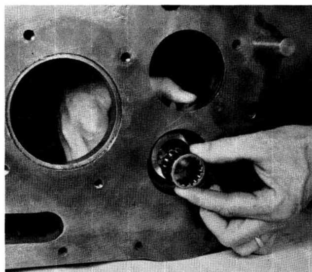
104. Installing needle bearing in hub of reverse-idler gear.
