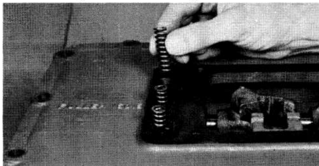
10. Removing the tension springs.
