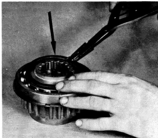
134. Installing bearing retaining snap ring in groove in drive gear shoulder.
