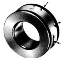
BALL DEPRESSIONS, CAUSED BY OFF-CENTER BLOW
