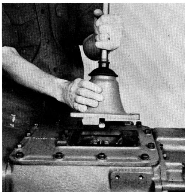
176. Installing the gear shift lever housing.
