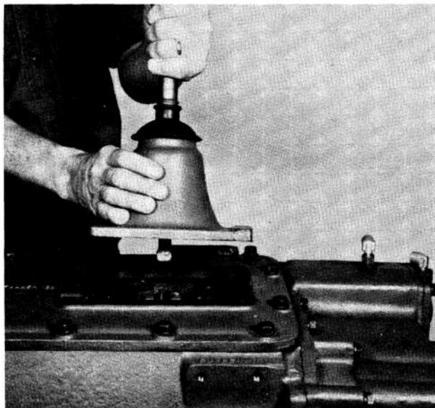
6. Removing the gear shift lever housing.
