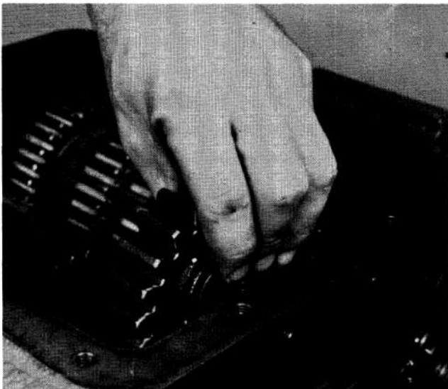
153. Placing reverse-idler gear into position in case.
