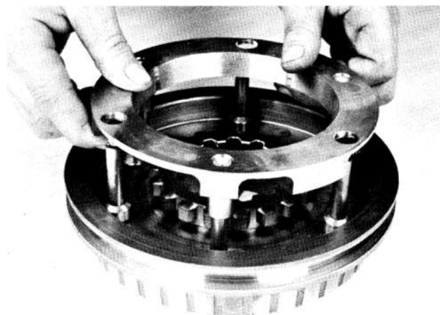
83. Placing high range synchronizer ring over pins of low speed synchronizer ring.
