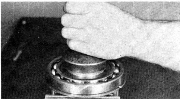
36. Driving auxiliary drive gear from bearing.
