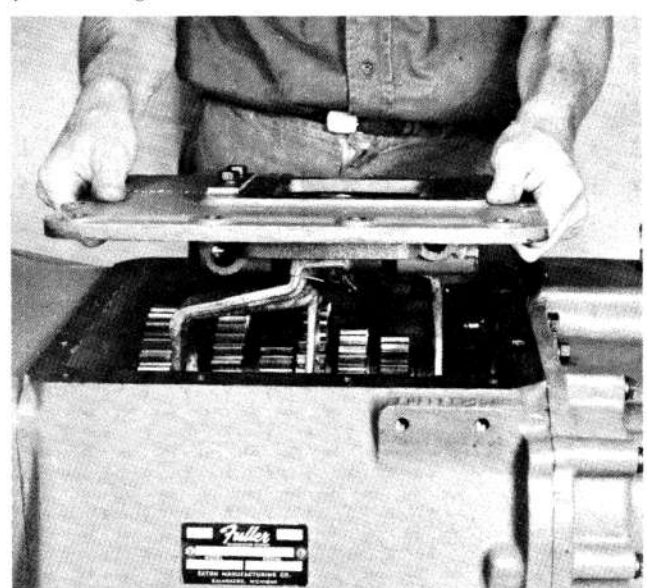
9. Lifting the shifting bar housing from transmission.
