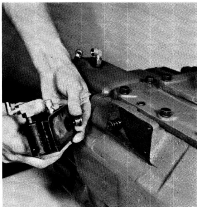
178. Installing the alignment sleeve in air valve.
