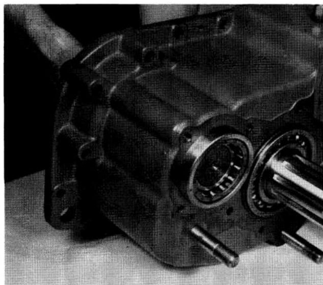
97. Placing countershafts into position in housing. At the same time, mesh timing tooth on each countershaft between timing teeth of low speed gear.
