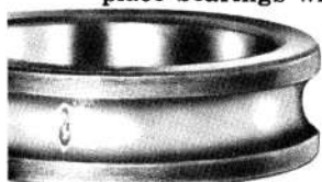
SPALLED BEARING — EXTREME LOAD
