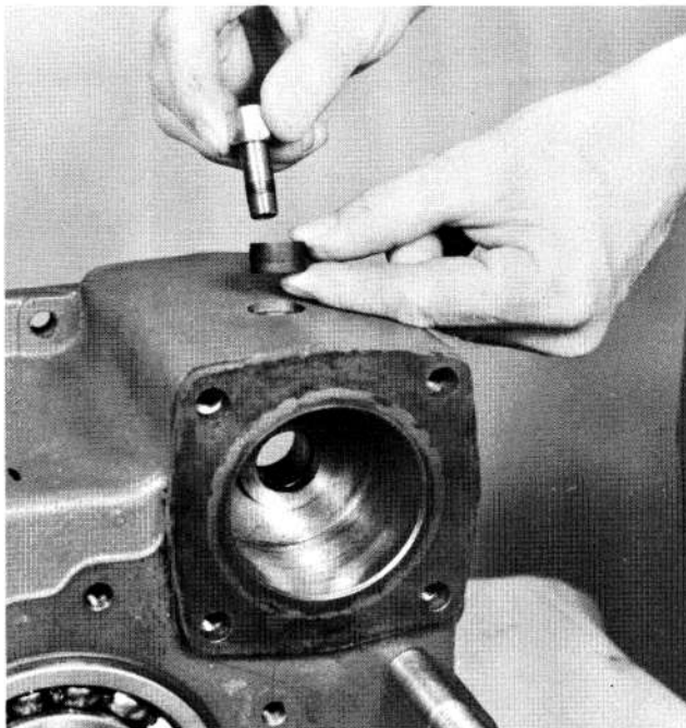
68. Removing the extension and dust seal from housing.
