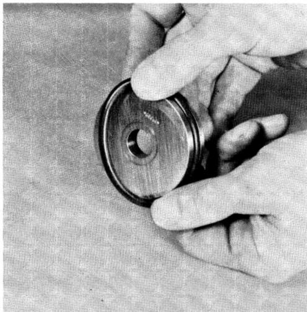
88. Installing O-ring on OD of piston.
