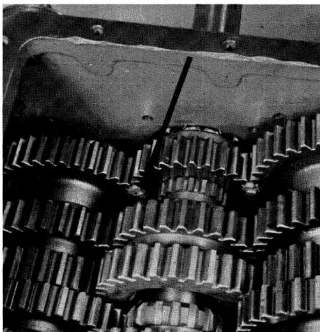
144. Left countershaft timing tooth meshed with timing teeth on drive gear.
