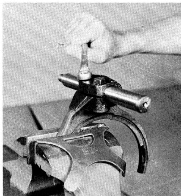
65. Removing shifting yoke from piston shaft.
