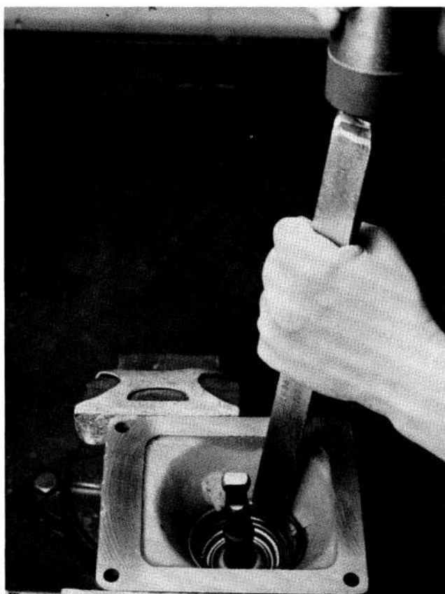
175. Installing the tension spring.
