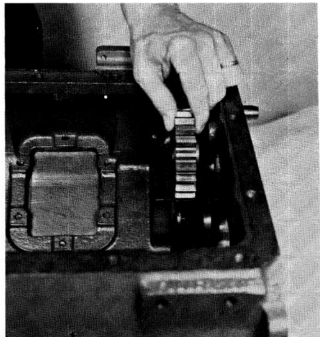
53. Removing the right reverse-idler gear from case.
