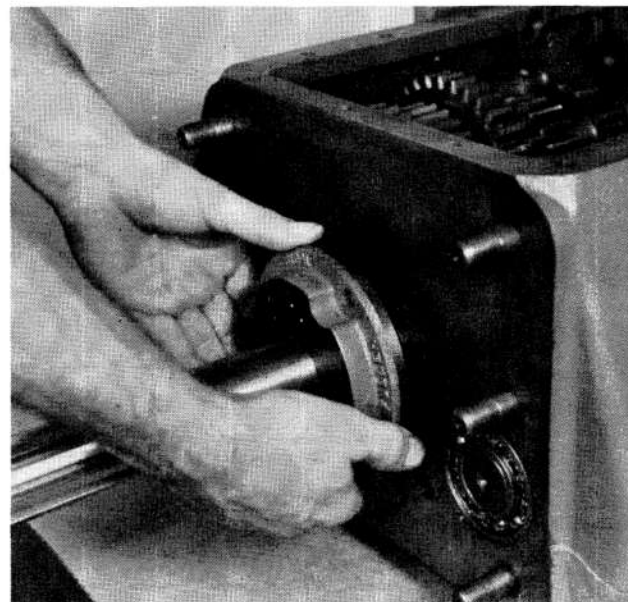
20. Removing the drive gear bearing cover.
