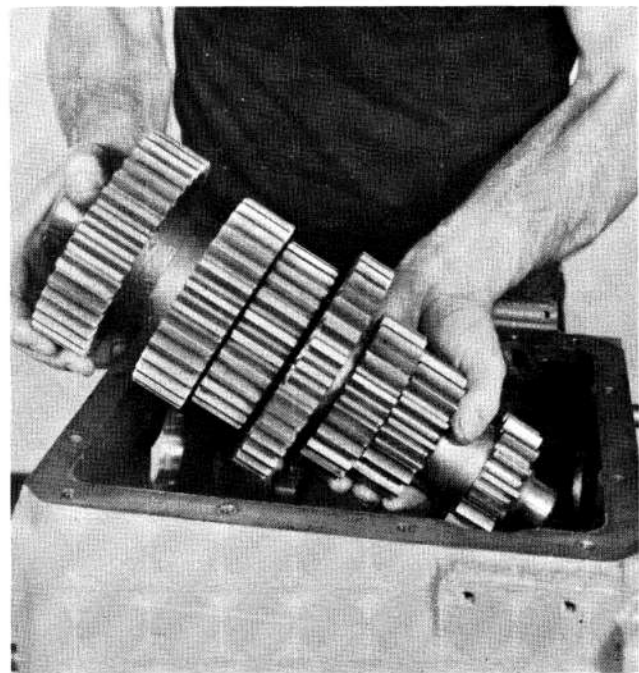
47. Lifting the left countershaft from case
